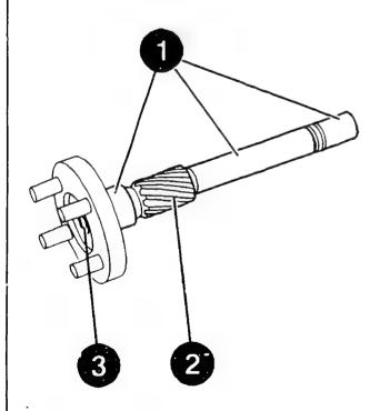
COMPONENT CHECKING AND REPAIR Checking planetary gear train Assembly: Prior to assembly, clean planetary gear train and remove both carbon brush abrasion and swarf. Lubricate in line with lubrication schedule during assembly. Slip TX collar (3) onto drive shaft (1). Insert drive shaft in intermediate bearing (2). Grease VS 16069-Ft: 5 984 610 120
